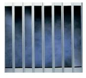
Curtain: 7" (178 mm) standard-width panels with 1/8" (3 mm) thick tempered glass that fit into aluminum hinges. Panels are framed by min. 4" (102 mm) high aluminum bottom plates and 5 1/4" (133 mm) high aluminum top plates.
