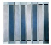
Curtain: 7" (178 mm) standard-width, 18-gauge painted perforated steel panels with 3/16" (5 mm) dia. holes on staggered centers that slide into aluminum hinges. Panels are framed by min. 4" (102 mm) high aluminum bottom plates and 5 1/4" (133 mm) high aluminum top plates. Visibility: 51% of 4 3/4" (121 mm) viewable area.
