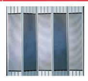
Curtain: 11 1/4" (286 mm) wide-body panels, constructed of 18-gauge painted perforated steel with 3/16" (5 mm) dia. holes on staggered centers that slide into aluminum hinges. Panels are framed by min. 4" (102 mm) high aluminum bottom plates and 5 1/4" (133 mm) high aluminum top plates. Visibility: 51% of 8 7/8" (225 mm) viewable area.
