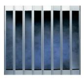
Curtain: 7" (178 mm) standard-width panels with 1/8" (3 mm) thick fire-retardant polycarbonate that fit into aluminum hinges. Panels are framed by min. 4" (102 mm) high aluminum bottom plates and 5 1/4" (133 mm) high aluminum top plates. Visibility: 100% of 4 3/4" (121 mm) viewable area\*.
