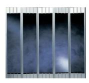
Curtain: 11 1/4" (286 mm) widebody panels with 1/8" (3 mm) thick fire-retardant polycarbonate that fit into aluminum hinges. Panels are framed by min. 4" (102 mm) high aluminum bottom plates and 5 1/4" (133 mm) high aluminum top plates. Visibility: 100% of 8 7/8" (225 mm) viewable area\*
